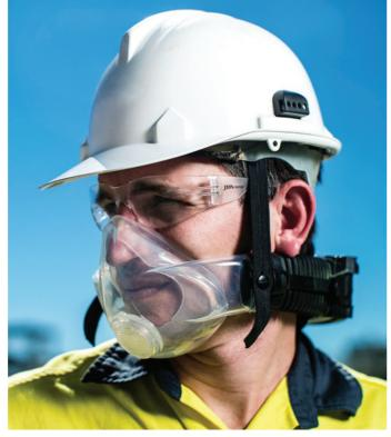
**SAFE** Fully certified positive pressure respirator with P3 TM3 filtration efficiency ensuring maximum protection in the workplace. Full Face Visor is high impact rated. Breath responsive. Up to 8 hours run time (Lithium polymer battery allows top up charging for a 12 hrs shift). TSI Portacount fit testing enabled. Particulate (P3) and combination gas filters available.
