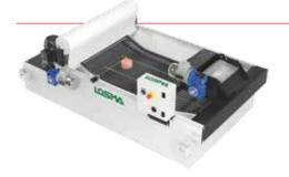
Flatbed filter for neat oil and emulsion filtration, contaminated by both magnetic and non-magnetic particles. Available in 8 different models with flow rates from 15 to 200 l/min of neat oil and from 30 to 400 l/min of emulsion, it can be equipped with fabrics with different filtration degrees (efficiency from 50 to 10 microns). Also available in stainless steel for filtering process requested for the chemical, food and class industry.
